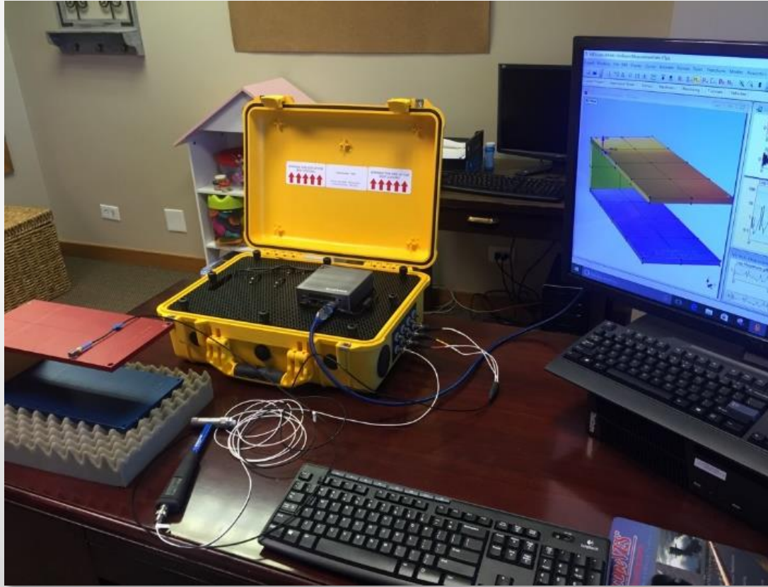
Impact Test with Roving Tri-Axial Accel
