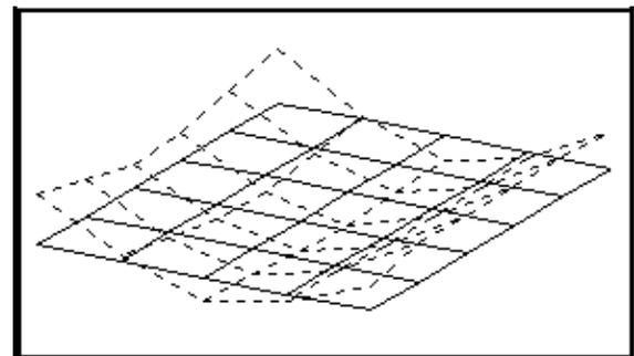
Figure 6. Operating Deflection Shape from FRFs at 765 Hz.
