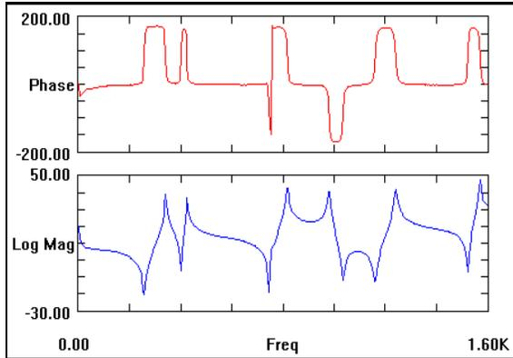
Figure 1. An FRF Measurement.
