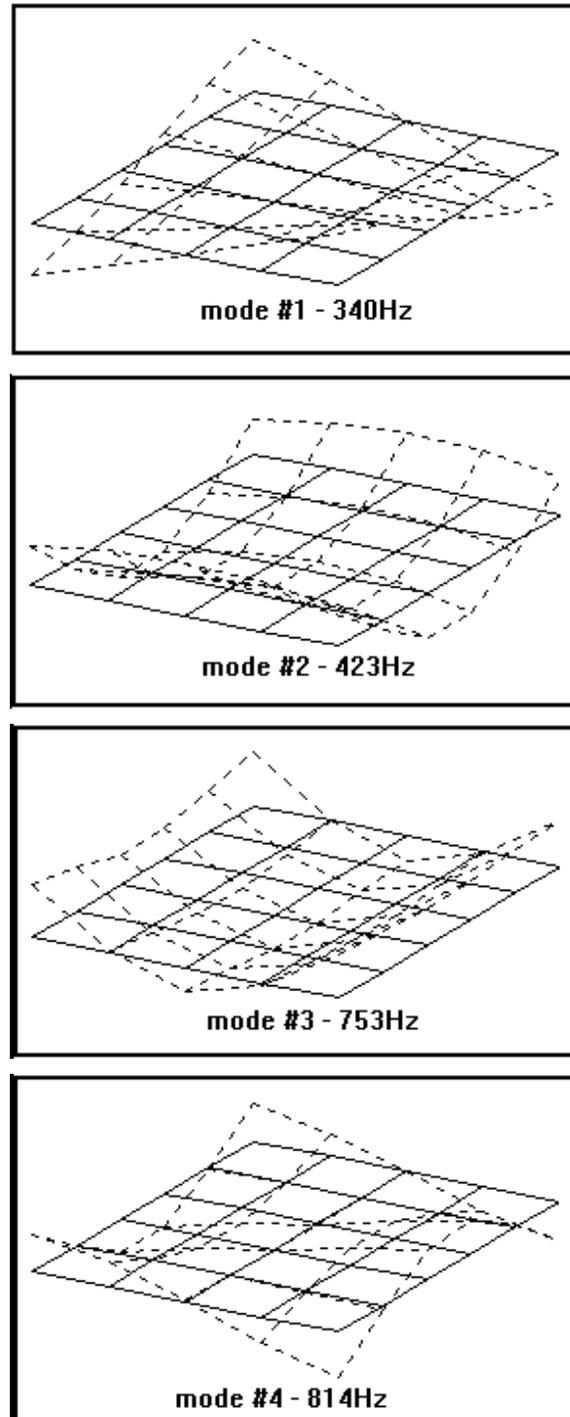
Figure 3. Mode Shapes of the Fundamental Modes.
