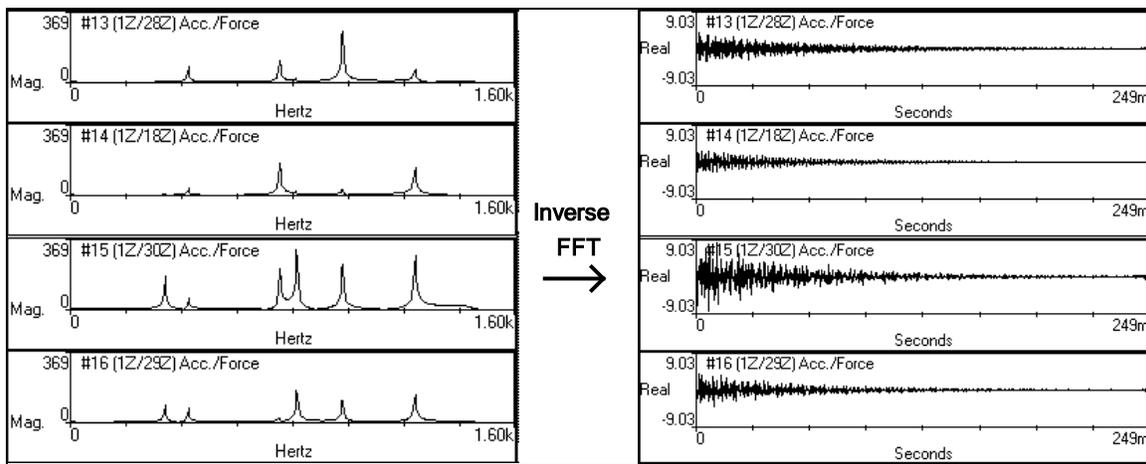
Figure 2. FRF Measurements and Corresponding Impulse Responses.
