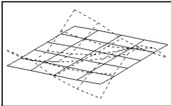
Figure 7. Operating Deflection Shape from FRFs at 785 Hz.
