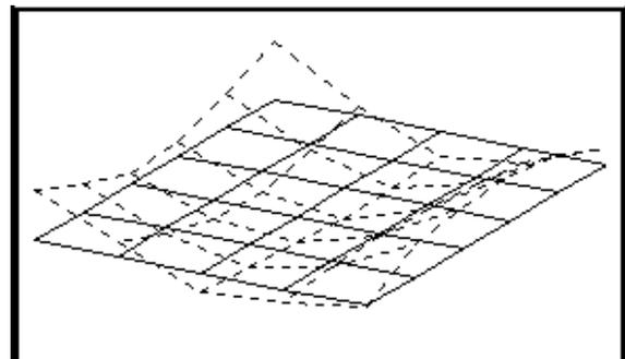
Figure 5. Operating Deflection Shape from FRFs at 780 Hz.
