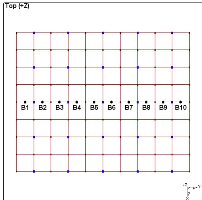
Figure 6. Top View of Plate Showing Bar Elements.
