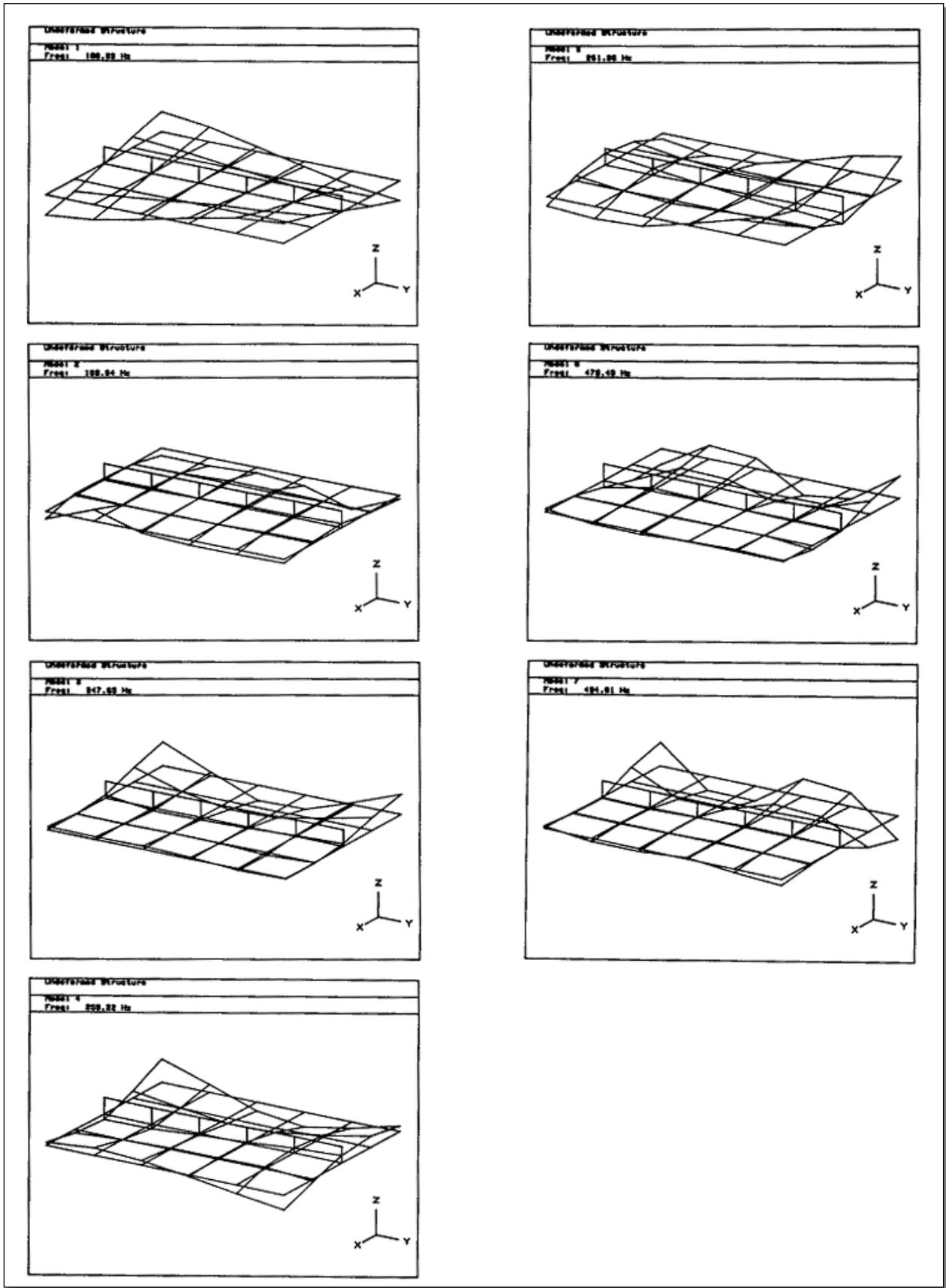
Figure 10. Mode Shape Differences Before and After End Bolt Removed
