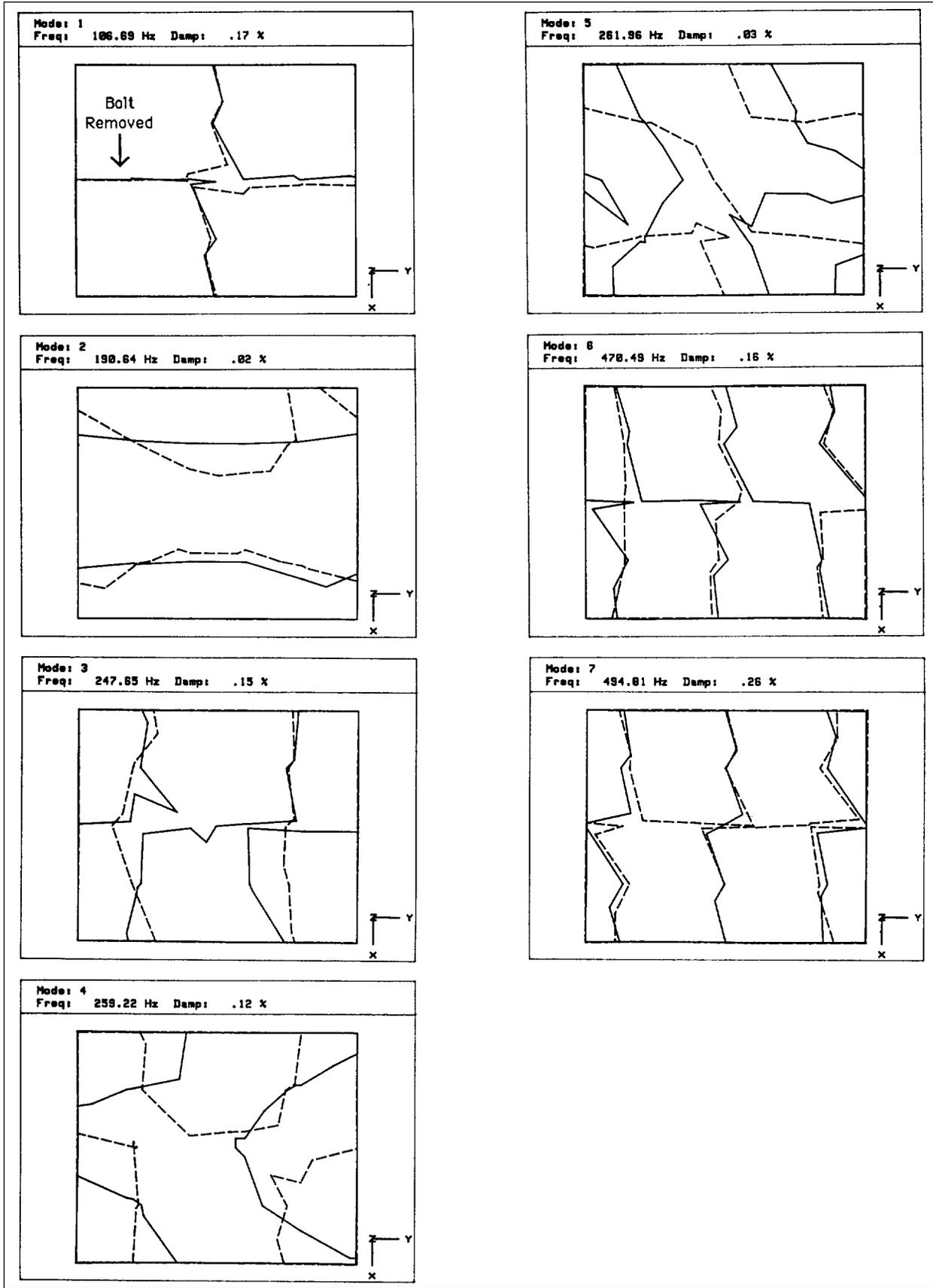
Figure 11. Mode Shape Node Lines Before and After End Bolt Removed
