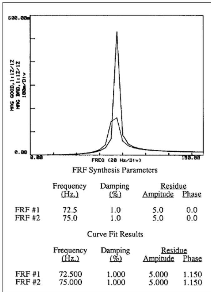
Figure 2. Curve Fir of Low Resolution FRFs
