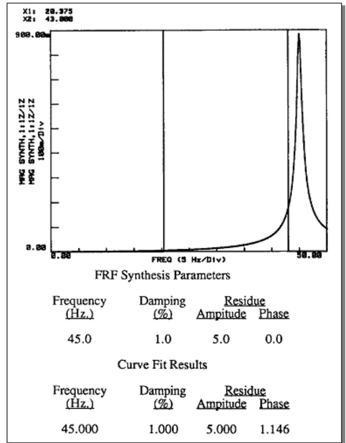
Figure 3. Curve Fit of FRF Away from Resonance
