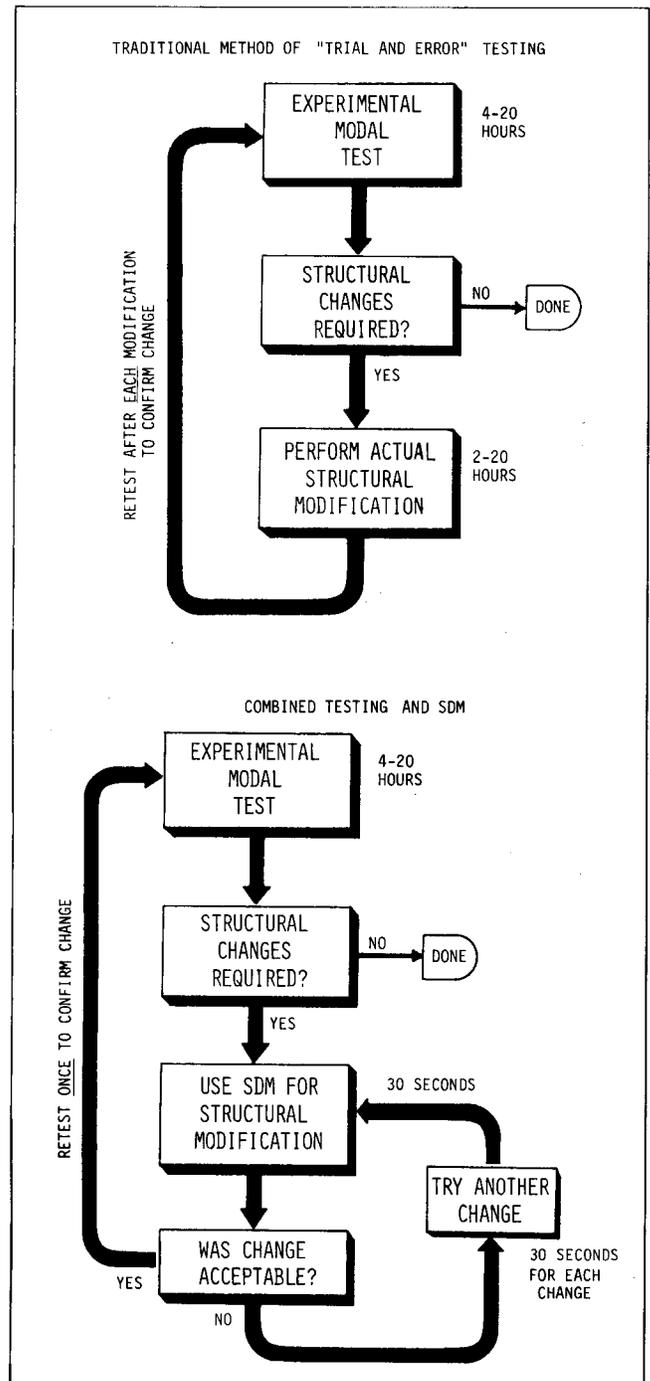
Figure 7. Procedures for troubleshooting noise and vibration problems.
