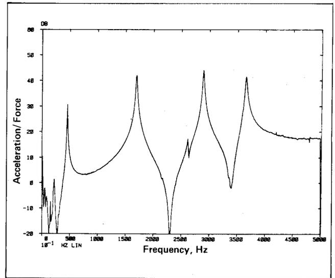
Figure 2. Frequency response measurement to identify structural resonances.
