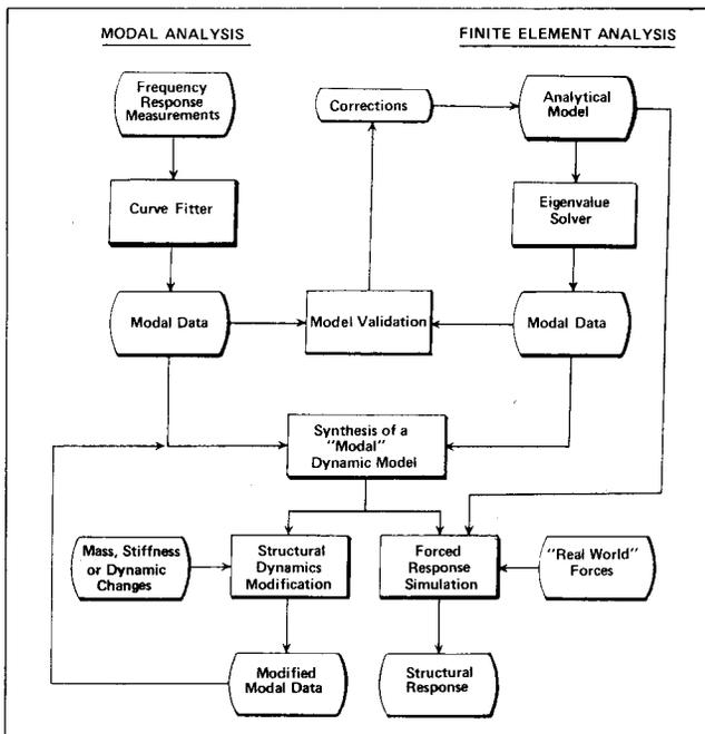
Figure 6. Combined testing and analysis techniques.
