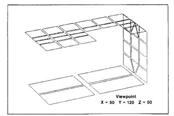
Figure 12. FEM mesh grid.
