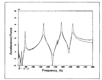
*Figure 3. The effect of adding damping to reduce the dynamic response of a structure at resonance.*
