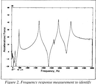
Figure 2. Frequency response measurement to identify structural resonances.
