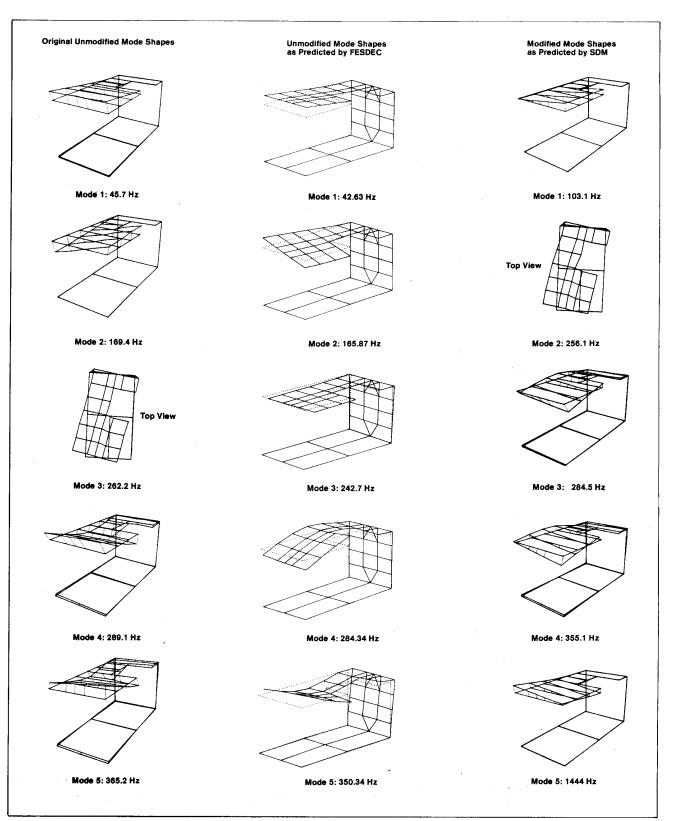
Figure 13. Comparison of mode shapes.
