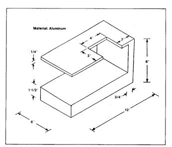
Figure 9. SDM/FESDEC test structure.
