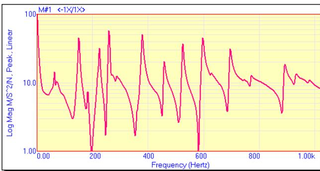
Figure 6. FRF With High Q Resonance Peaks.
