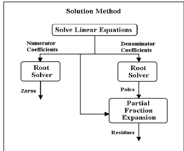
Figure 23. RFP Solution Method.
