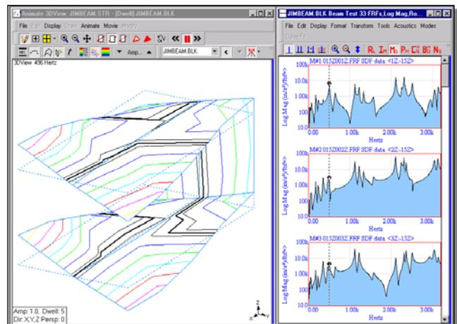
Figure 1. Frequency Domain ODS From a Set of FRFs
