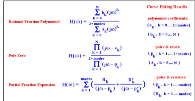
Figure 22. Alternate Curve Fitting Forms of the FRF.
