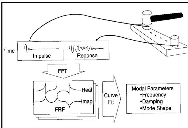
Figure 9. Impact Testing.
