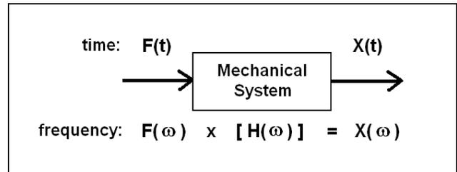
Figure 3. Block Diagram of an FRF.
