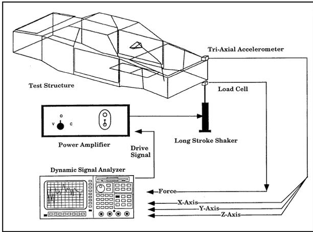
Figure 11. Shaker Test Setup.
