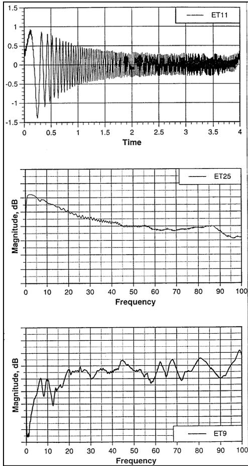
Figure 14. Burst Chirp Excitation (Time waveform, APS, FRF & Coherence)
