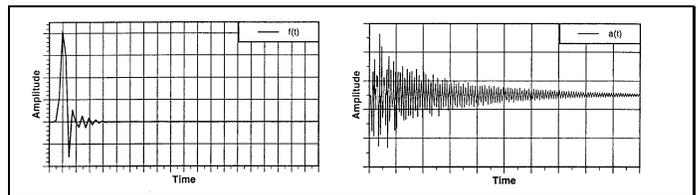
Figure 10A. Impact Force and Response Signals
