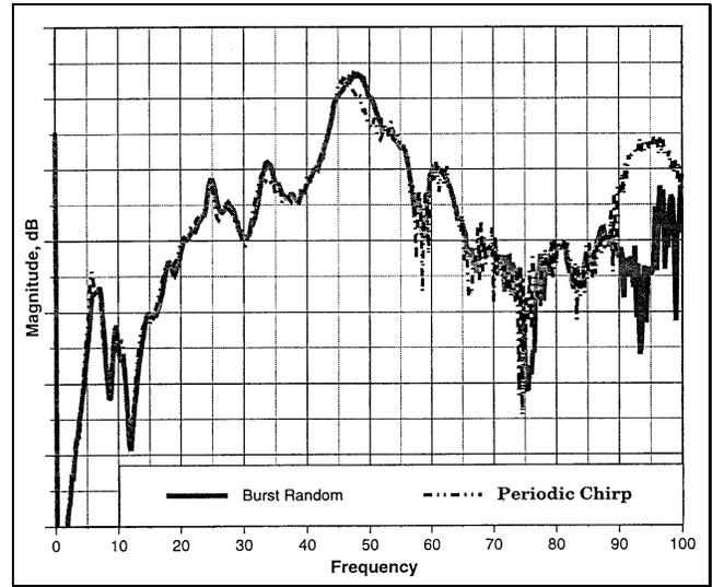
Figure 15. Burst Random Versus Burst Chirp FRF.
