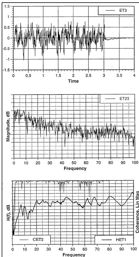
Figure 13. Burst Random Excitation (Time waveform, APS, FRF & Coherence).
