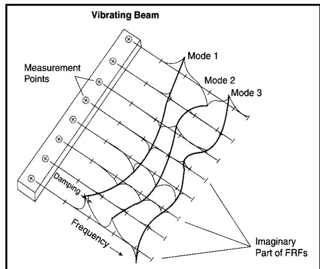
Figure 20. Curve Fitting FRF Measurements.
