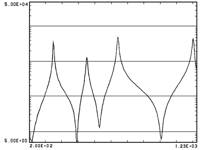
Figure 3. Circular Plate Test Structure Driving Point FRF
