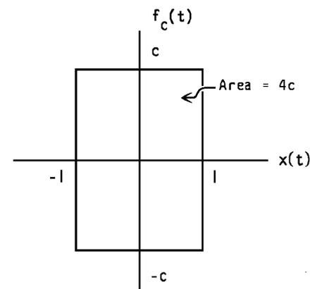
Figure 2. Hysteresis Curve for Coulomb Damping
