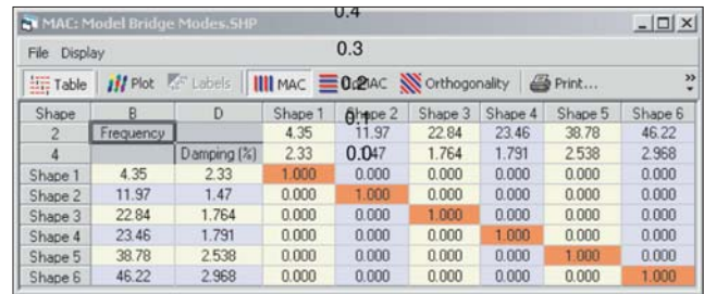
Figure 23: MAC matrix using 175 DOF FEA model.
