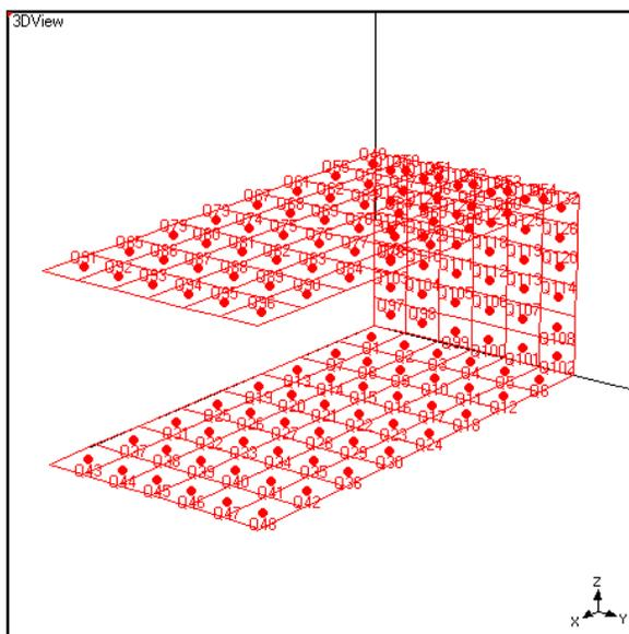
Figure 2. FEA Model with 132 Quad Plate Elements.
