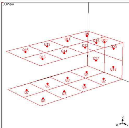
Figure 4. FEA Model with 20 Quad Plate Elements.
