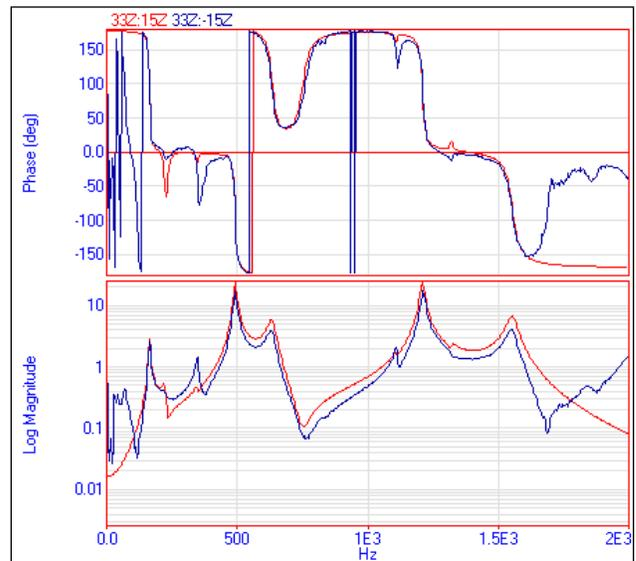
Figure 3B Overlaid Synthesized and Measured FRFs Between Top & Back Plate.
