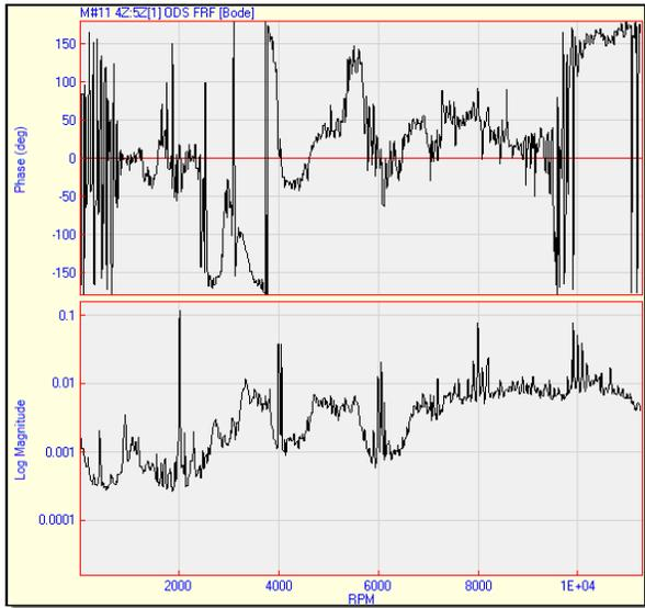
Figure 2. ODSFRF Showing Peaks at Machine Orders.
