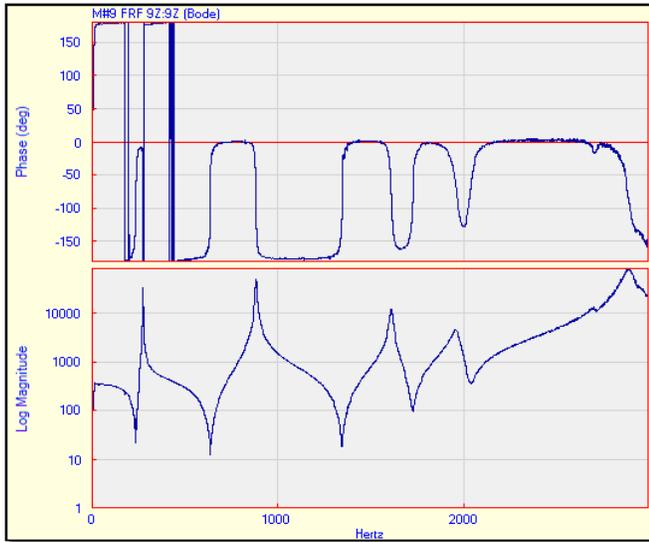
**Figure 2. Typical FRF Measurement**
