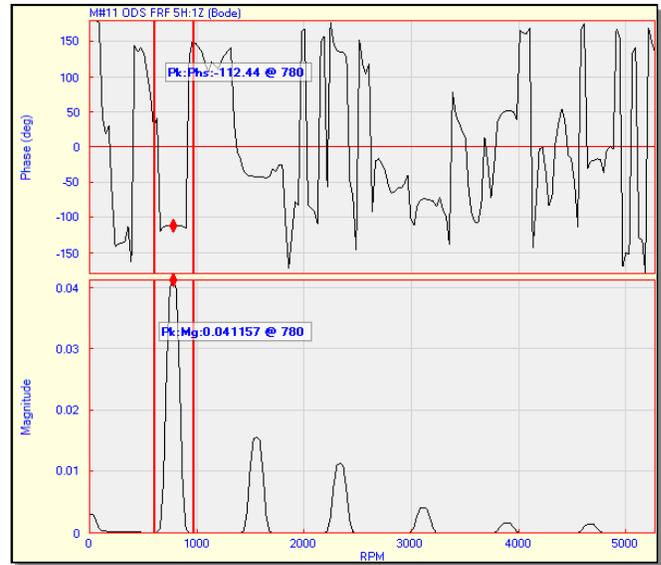
Figure 3 ODSFRF Showing Peaks at Machine Orders
