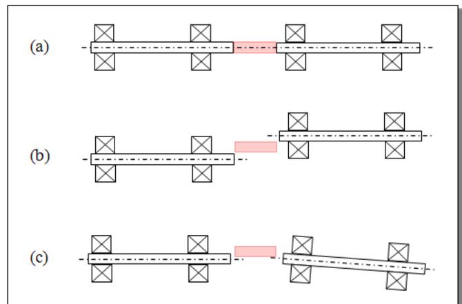
Figure 4. Parallel and Angular Misalignment
