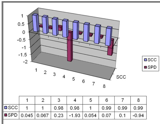
**Figure 8. Parallel Misalignment ODS Comparisons**
