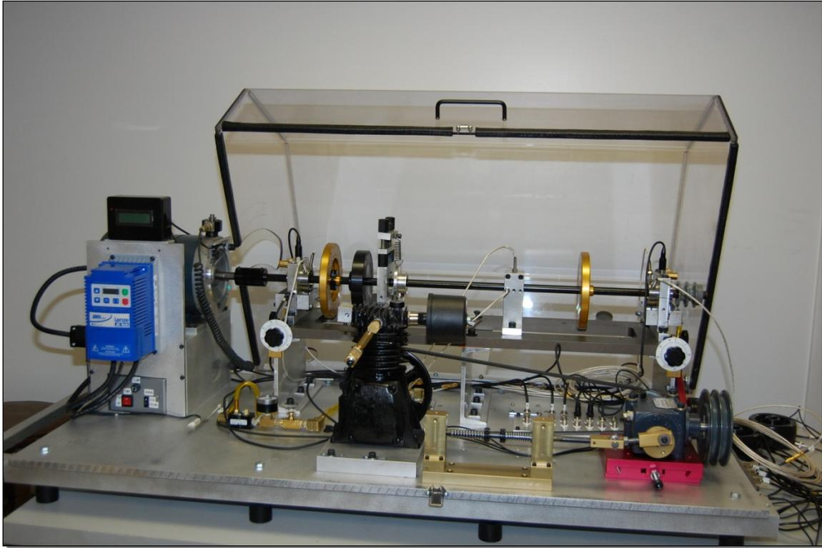
*Figure 1. Machine Fault Simulator*
