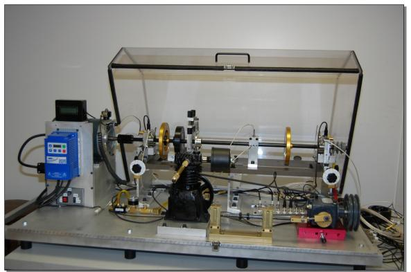
Figure 1. Machine Fault Simulator
