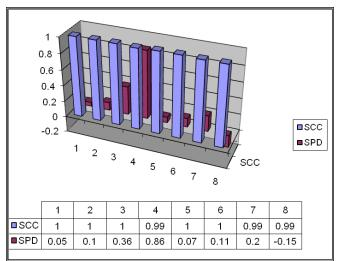
Figure 7. Angular Misalignment ODS Comparisons
