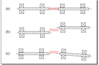
Figure 4. Parallel and Angular Misalignment
