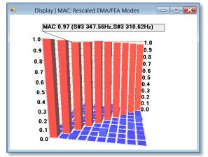
Figure 7. MAC Values Between Rescaled EMA & FEA Shapes
