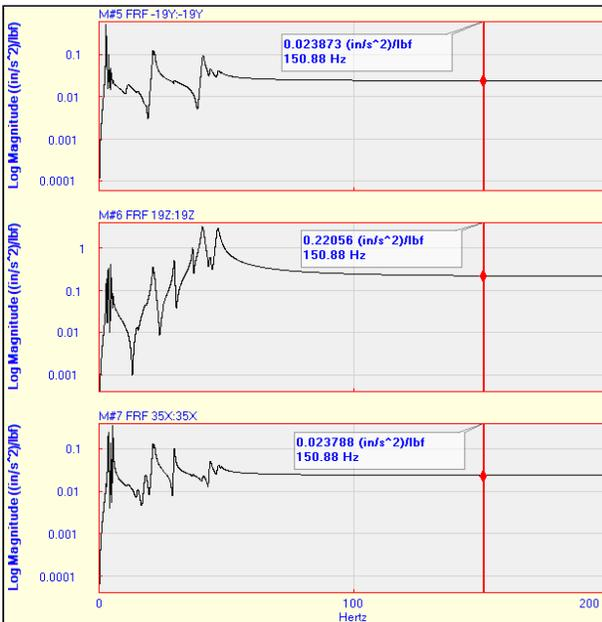
Figure 5 Inertance Mass Line ( $\text{in}/\text{sec}^2\text{-lbf} = 1/\text{mass}$ ).
