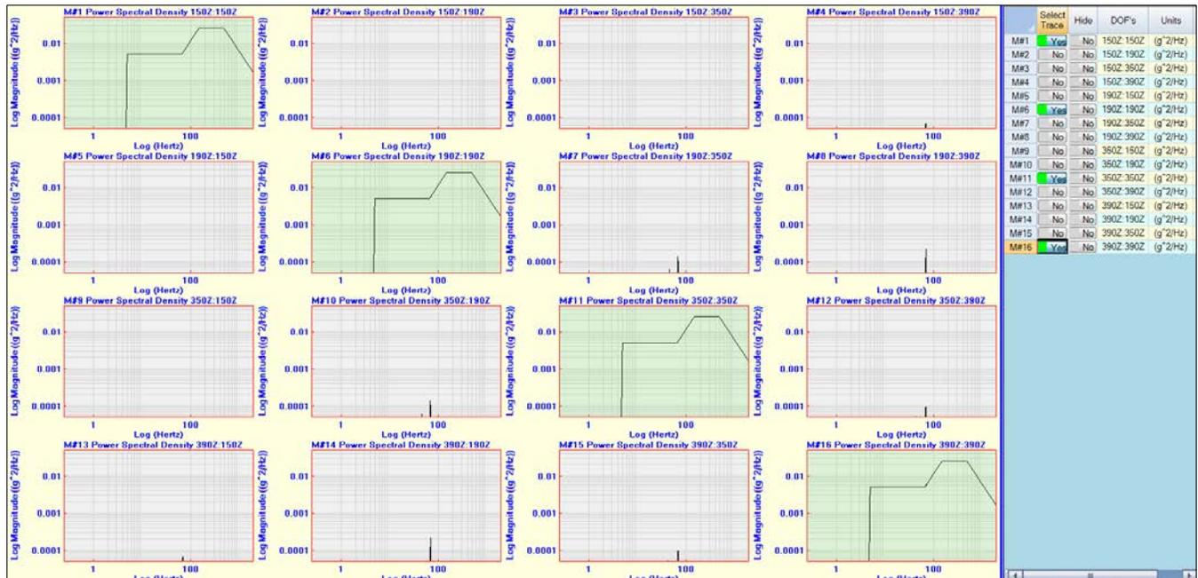
Figure 10 C-17 Simulated Base-Shake PSDs.
