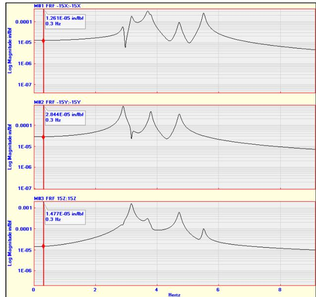
Figure 3 Flexibility Line at Low Frequency (in/lbf = 1/Stiffness)
