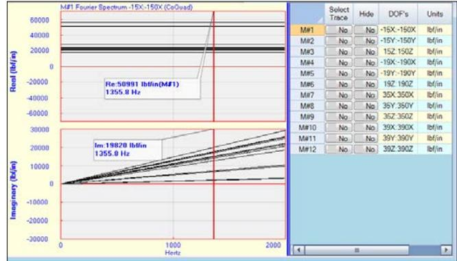
Figure 6 Stiffness & Damping matrix.
