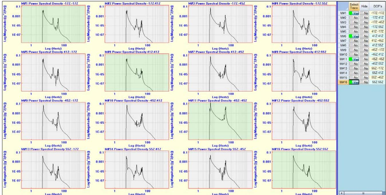
Figure 9 C-17 Control PSDs for 4 Z-direction Driving Points.
