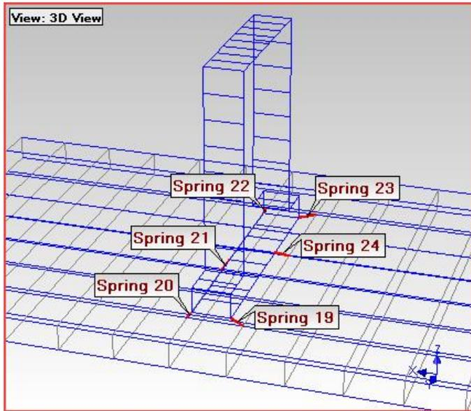
Figure 8. Springs Connecting Base Plate & Bearing Blocks.
