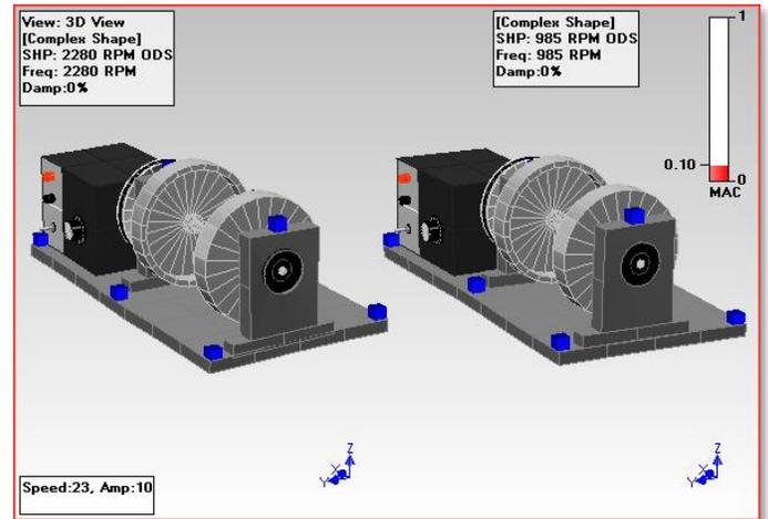
Figure 5. ODSs at 985 & 2280 RPM.
