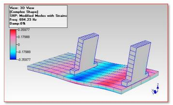
Figure 7C. Normal Strain, X-Direction, Mode #10.
