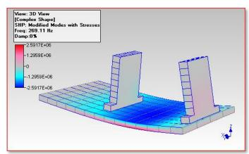
Figure 8A. Normal Stress, X-Direction, Mode #7.
