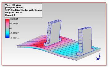
Figure 7B. Normal Strain, X-Direction, Mode #9.
