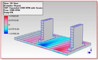
Figure 9B. Normal Strain, X-Direction, 2280 RPM ODS.
