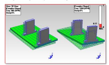
Figure 6. Expanded ODS's of Base Plate & Bearing Blocks.
