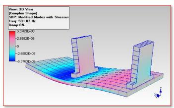
Figure 8B. Normal Stress, X-Direction, Mode #9.
