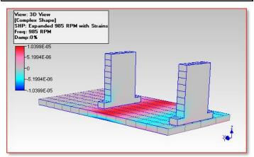
Figure 9A. Normal Strain, X-Direction, 985 RPM ODS.
