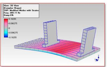
Figure 7A. Normal Strain, X-Direction, Mode #7.
