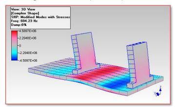
Figure 8C. Normal Stress, X-Direction, Mode #10.
