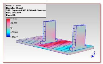
Figure 10A. Normal Stress, X-Direction, 985 RPM ODS.
