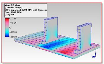
Figure 10B. Normal Stress, X-Direction, 2280 RPM ODS.
