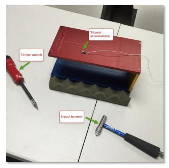
Figure 1. Jim Beam Test Structure.
